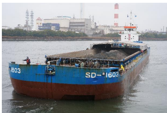
Photo 2-10 Ship to Transport Waste (The roof is closed after departure to prevent waste scattering)
