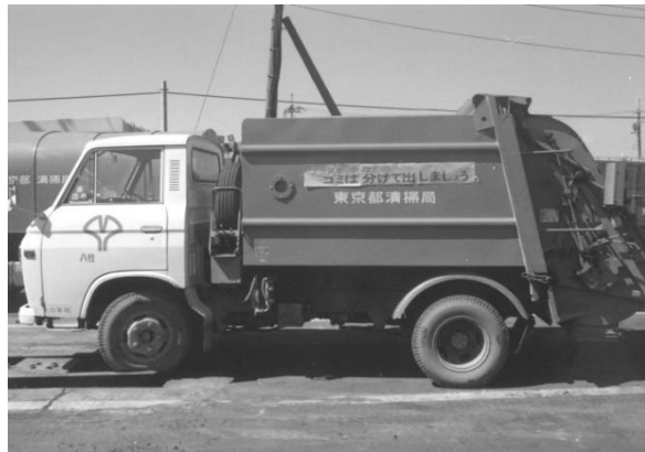
Source: Tokyo Metropolitan Government Bureau of Environment Photo 2-6 Collection Vehicle with Compaction Function (Compacter)
